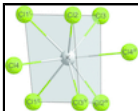
Fig. 2. Coordination sphere of the K + cations with the shape of a bicapped trigonal prism. [Symmetry codes: (i) -x+1/2, -y+1, z-1/2 ; (ii) x+1/2, y, -z+3/2 ; (iii) -x+3/2, -y+1, z+1/2 ; (iv) -x+3/2, -y+1, z-1/2 .]
